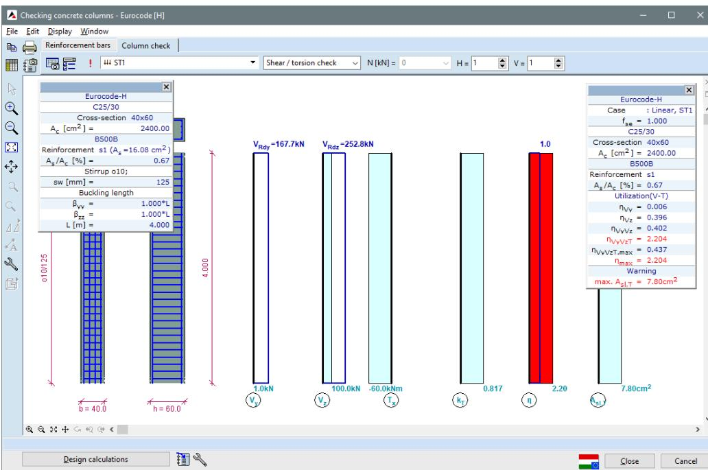
The screenshot shows the AxisVM software interface for concrete column verification. The main window displays a 3D model of a rectangular concrete column with dimensions b=40.0 and h=60.0. The reinforcement bars are shown as blue vertical bars. The software interface includes several input parameters and calculated values:
