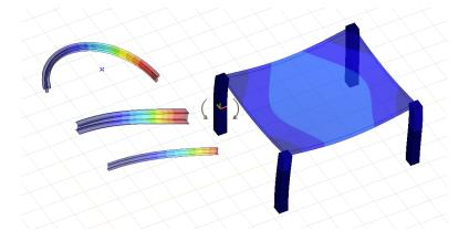
Rendered view can display distribution of normal stress within the cross-section of a beam
