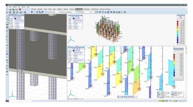
• Calculation of the required reinforcement for reinforced trapezoid steel decks. (**RC1** module)
