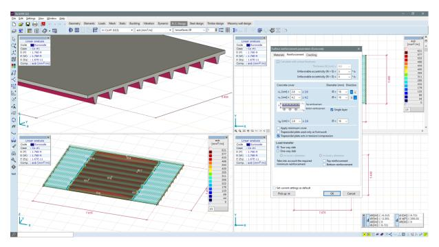
• New table for specific amount of reinforcement calculated for each domain (**RC1** module)
