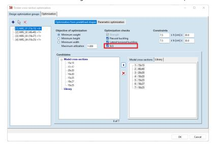
Replace cross sections of timber design members (TD1 module)
