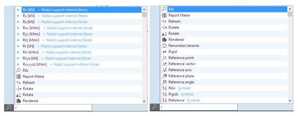
Additional functions are: finding an element by its number or name, selecting elements by property value (material, cross-section, length, eccentricity, domain thickness, domain area), by value of a result component, or by using multiple criteria.
