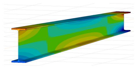
• Rendered view can display top and bottom components of surface stresses, reinforcement amounts, and crack width values simultaneously (**RC1** module)
